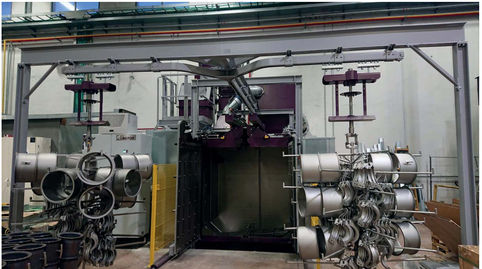
The AGTOS Hanger-type blast machine from type HT 17-17.
