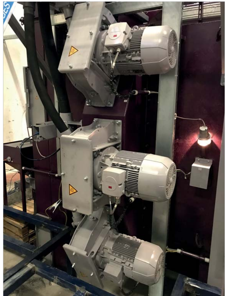
AGTOS turbines with wear parts made of highly wear-resistant hard metal.
